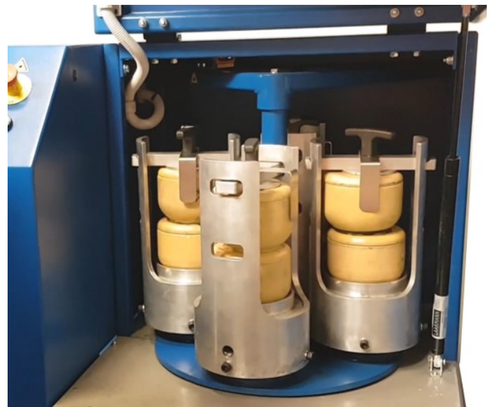
Planetary ball mill 8 grinding jar set up
